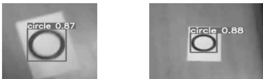
Figure 2. Successful object detection on a frame that was not part of the training set on Raspberry.
